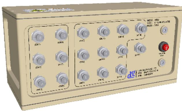
The DC Power Distribution Unit (PDU) distributes a single source DC supply to up to 17 connected devices. The DC PDU is designed to meet the rigorous requirements of Def-Stan 61-5 Part 6 Issue 6 and provides voltage surge, over-current and reverse polarity protection for all outputs as well as attenuation of conducted emissions above 1MHz.
