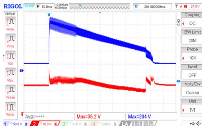
204Vpk pulse applied at input of the DC PDU suppressed to 35Vpk pulse at DC PDU outputs.
